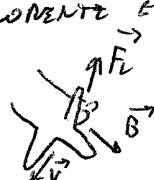
$$[\vec{B}] = \left[ \frac{\vec{F}_L}{q\vec{v}} \right] \Rightarrow T = \frac{N}{C \cdot s} = \frac{kg \cdot m/s^2}{C \cdot m/s} = \frac{kg}{C \cdot s}$$
