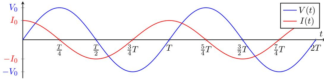
$$i(t) = C\omega V_0 \sin(\omega t + \frac{\pi}{2})$$
