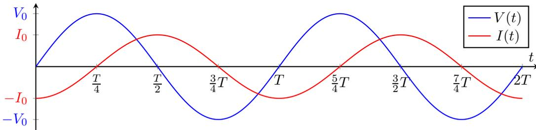
$$i(t) = -\frac{V}{\omega L} \cos \omega t = \frac{V_0}{\omega L} \sin(\omega t - \varphi) = 0 \frac{V}{\omega L} \sin\left(\omega t - \frac{\pi}{2}\right)$$
